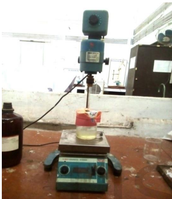
Figure.1. Experimental setup for kinetic studies (Stirred cell)
